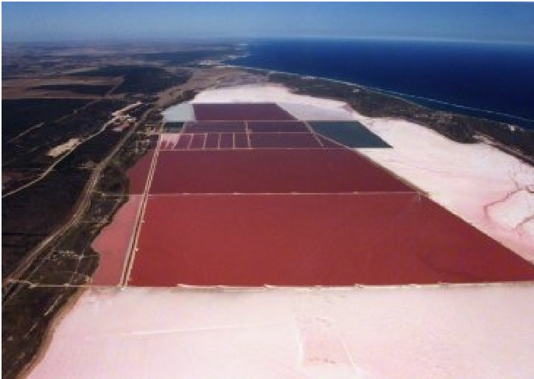
Figure 4. The large open ponds used for cultivating Dunaliella salina at Hutt Lagoon, Western Australia. 1
