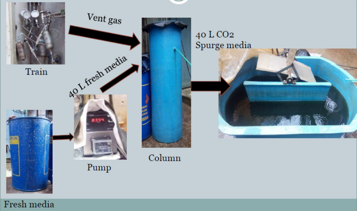
Figure 1: Carbon dioxide sequestration by algae experimental set up.
