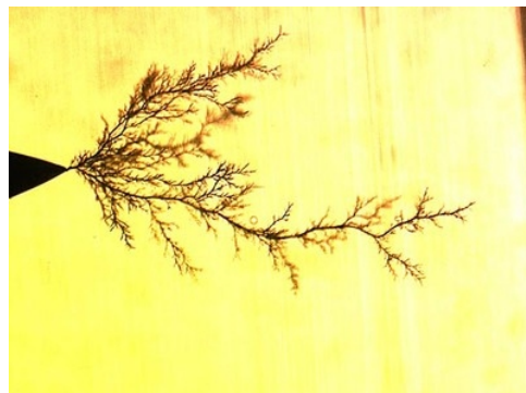
Figure 3.3. Branch-like electrical tree [32]
