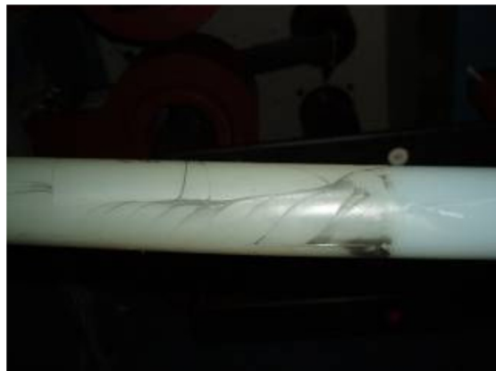
Figure 3.1. Surface tracking on top of insulation [25]
