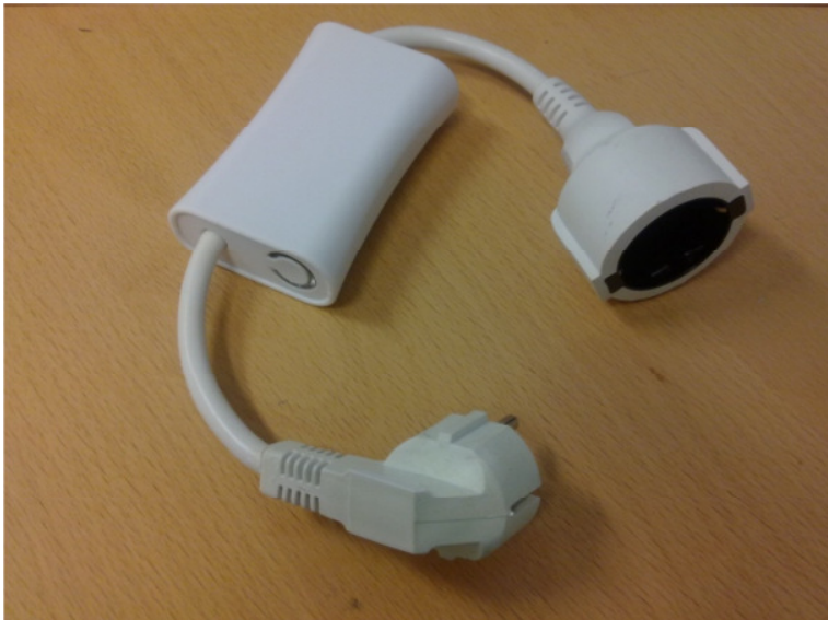
Figure 5.2. Smart Energy Switch, SES.
