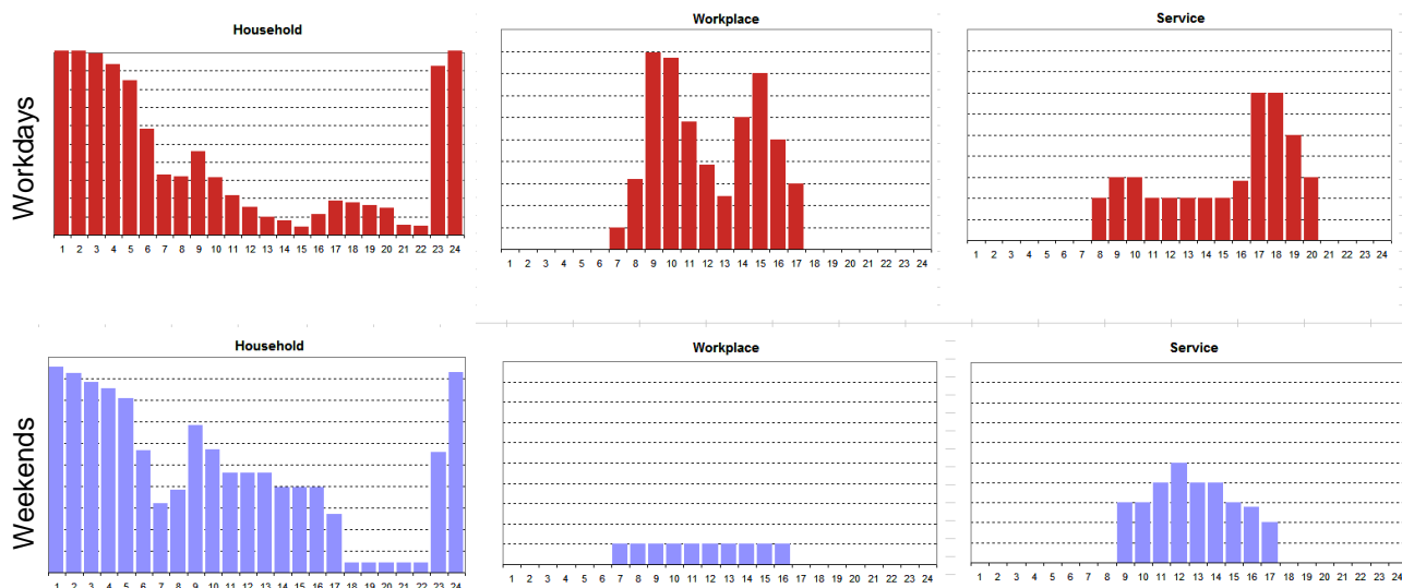
Figure 3. Three charging curves used in the study; households, workplaces and services on workdays and weekends.
