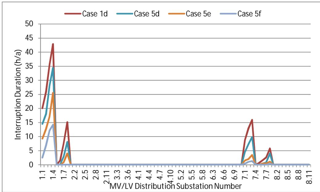
**Figure 5-24: Annual interruption duration for MV/LV substations (Case 5d-5f)**
