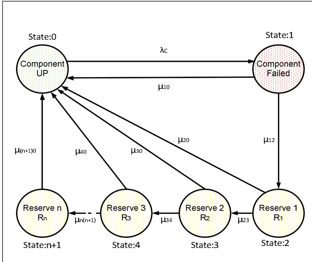
*Figure 4-2: Basic model for distribution network components.*
