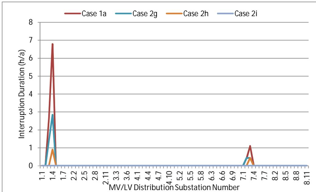
**Figure 5-13: Annual interruption duration for MV/LV substations (Case 2g-2i)**
