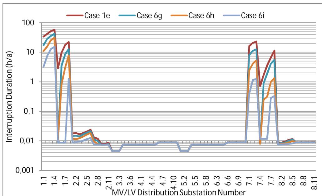
**Figure 5-29: Annual interruption duration for MV/LV substations (Case 6g-6i)**
