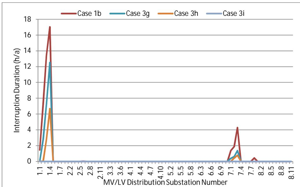
**Figure 5-17: Annual interruption duration for MV/LV substations (Case 3g-3i)**
