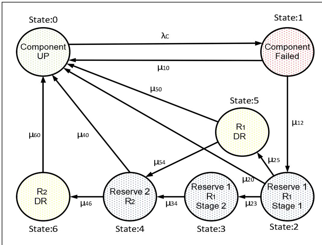
Figure 4-4: Modified model for HV/MV transformer.
