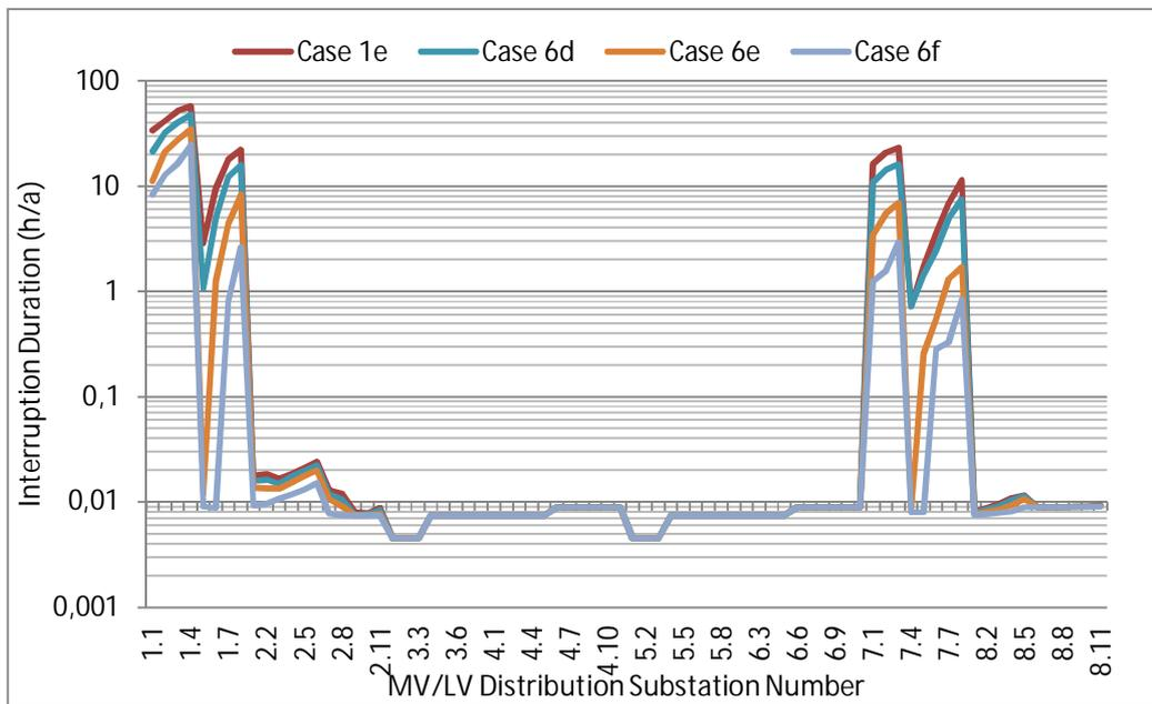
**Figure 5-28: Annual interruption duration for MV/LV substations (Case 6d-6f)**
