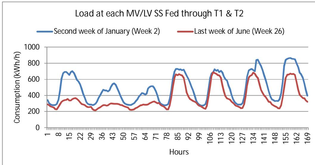
**Figure 5-3: Load profile of specific week at each MV/LV substation fed through T1 & T2.**
