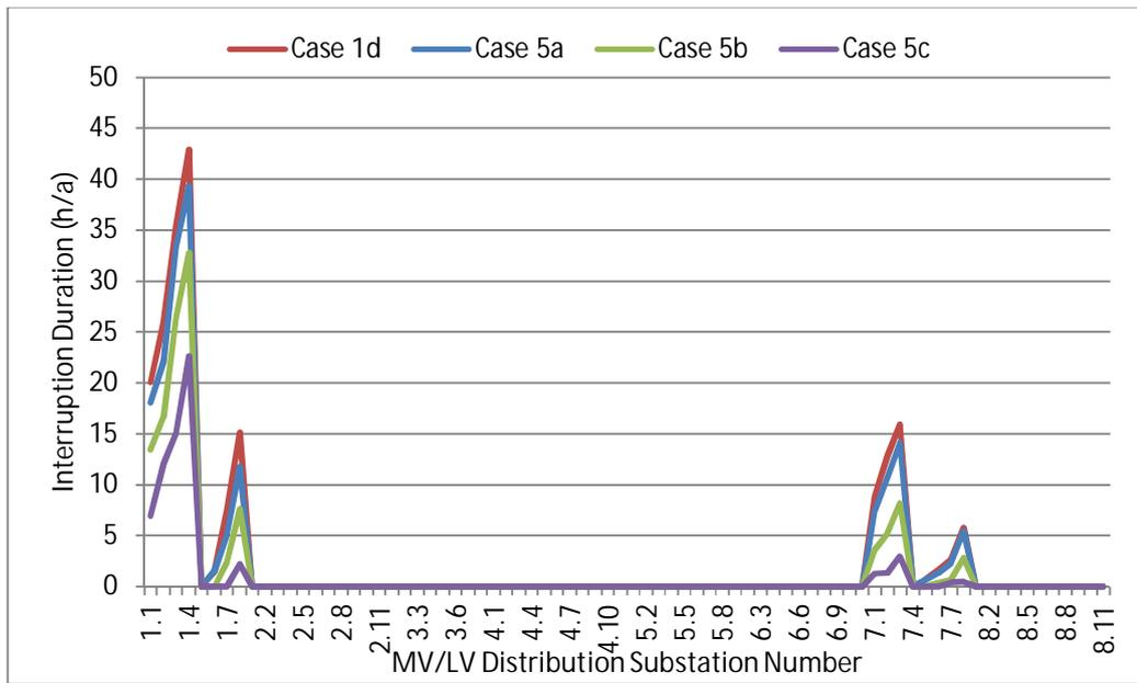
**Figure 5-23: Annual interruption duration for MV/LV substations (Case 5a-5c)**
