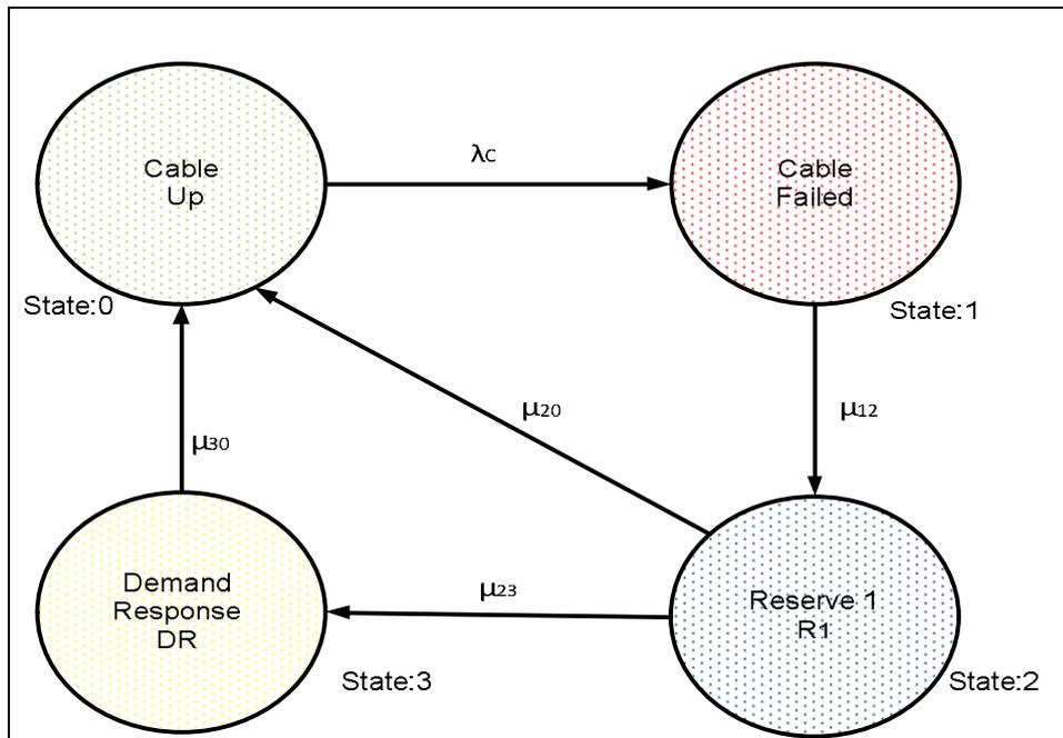
*Figure 4-5: Modified model for MV Cables.*
