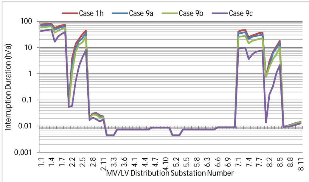
**Figure 5-39: Annual interruption duration for MV/LV substations (Case 9a-9c)**
