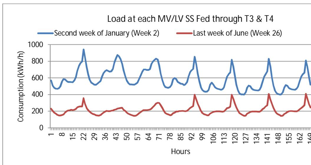
**Figure 5-5: Load profile of specific week at each MV/LV substation fed through T3 & T4.**
