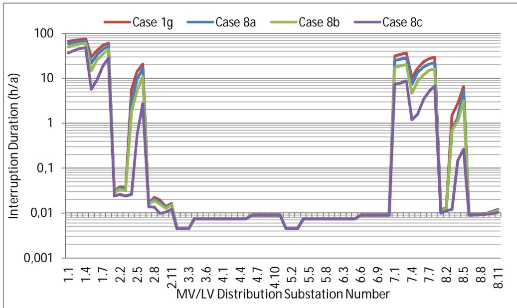
**Figure 5-35: Annual interruption duration for MV/LV substations (Case 8a-8c)**
