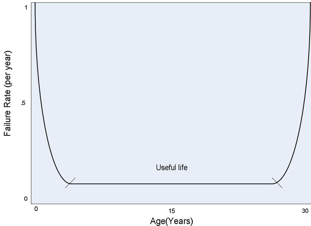
**Figure 3-1: Bathtub curve, failure rate character of many electrical components.**
