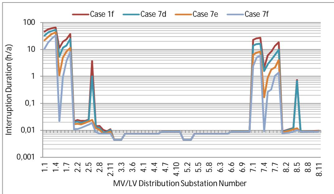
**Figure 5-32: Annual interruption duration for MV/LV substations (Case 7d-7f)**
