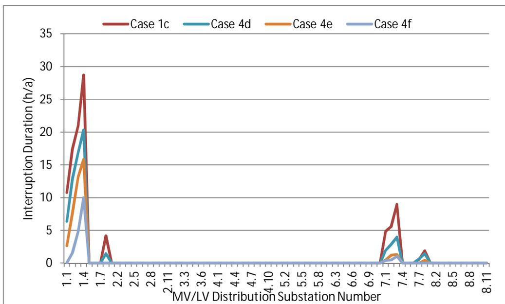
**Figure 5-20: Annual interruption duration for MV/LV substations (Case 4d-4f)**
