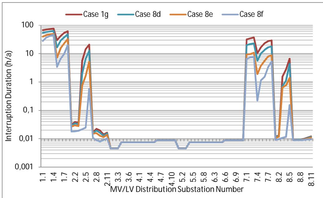
**Figure 5-36: Annual interruption duration for MV/LV substations (Case 8d-8f)**
