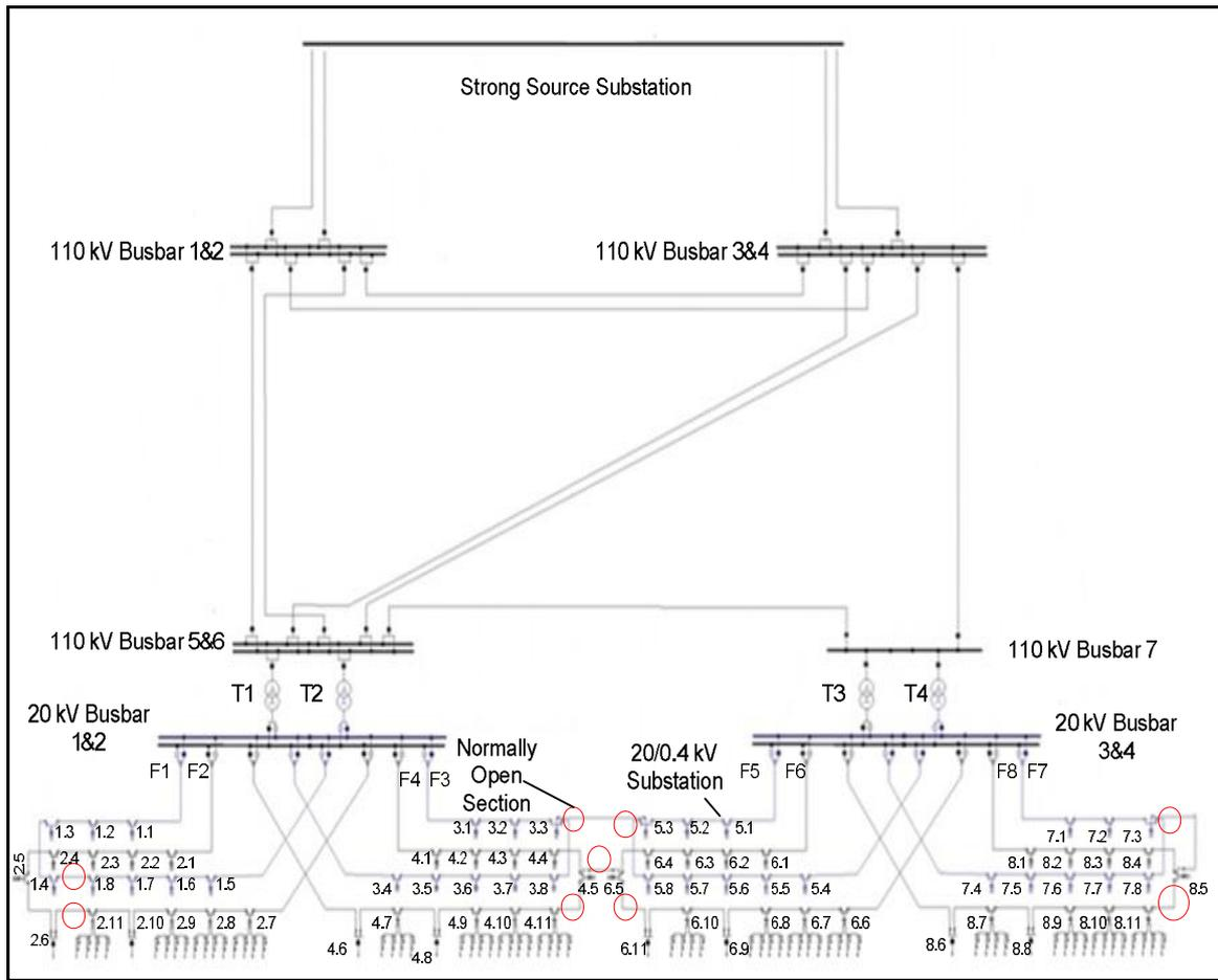
**Figure 5-1: Single-line diagram of typical Finnish sub-transmission (110kV) and primary distribution (20kV) network which is used as test network.**
