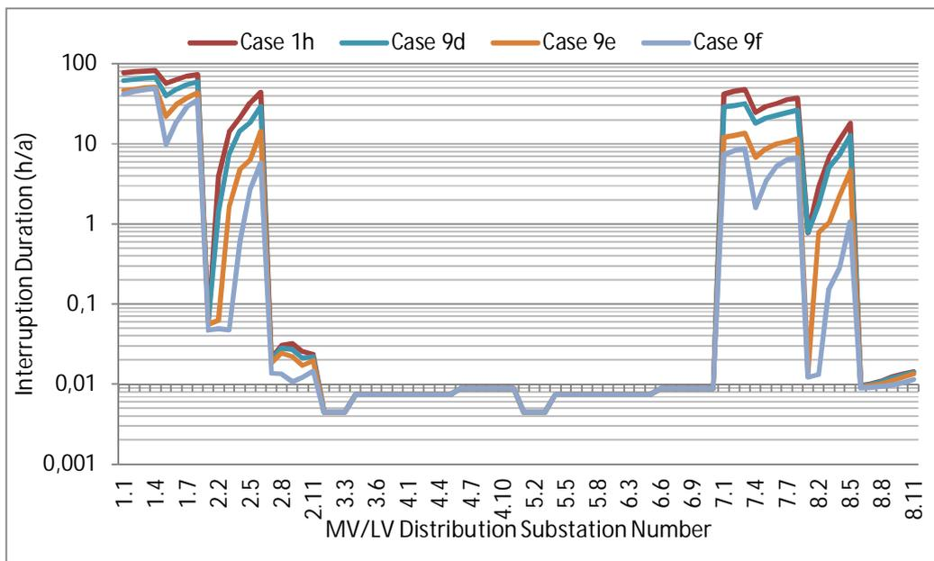
**Figure 5-40: Annual interruption duration for MV/LV substations (Case 9d-9f)**
