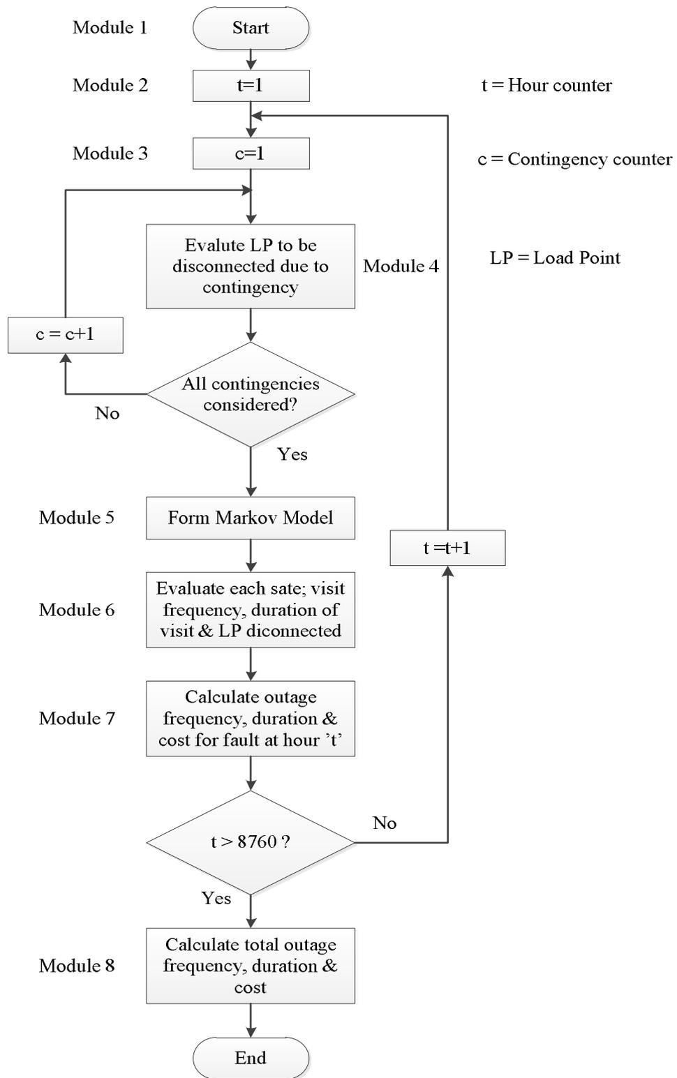
**Figure 4-6: Flow diagram for calculating reliability indices and total outage cost.**
