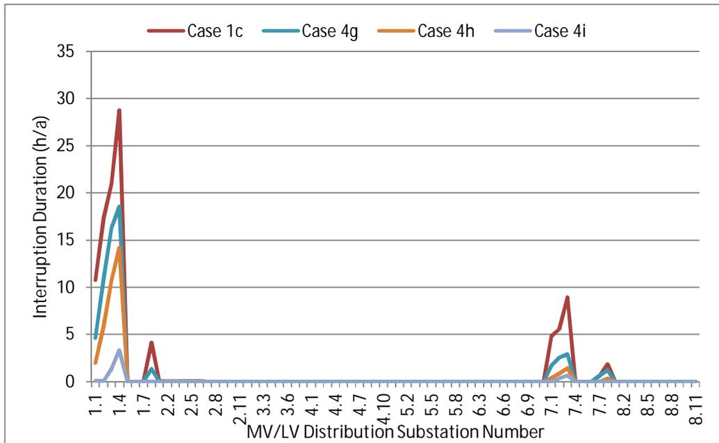
*Figure 5-21: Annual interruption duration for MV/LV substations (Case 4g-4i)*
