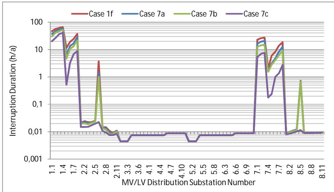
**Figure 5-31: Annual interruption duration for MV/LV substations (Case 7a-7c)**
