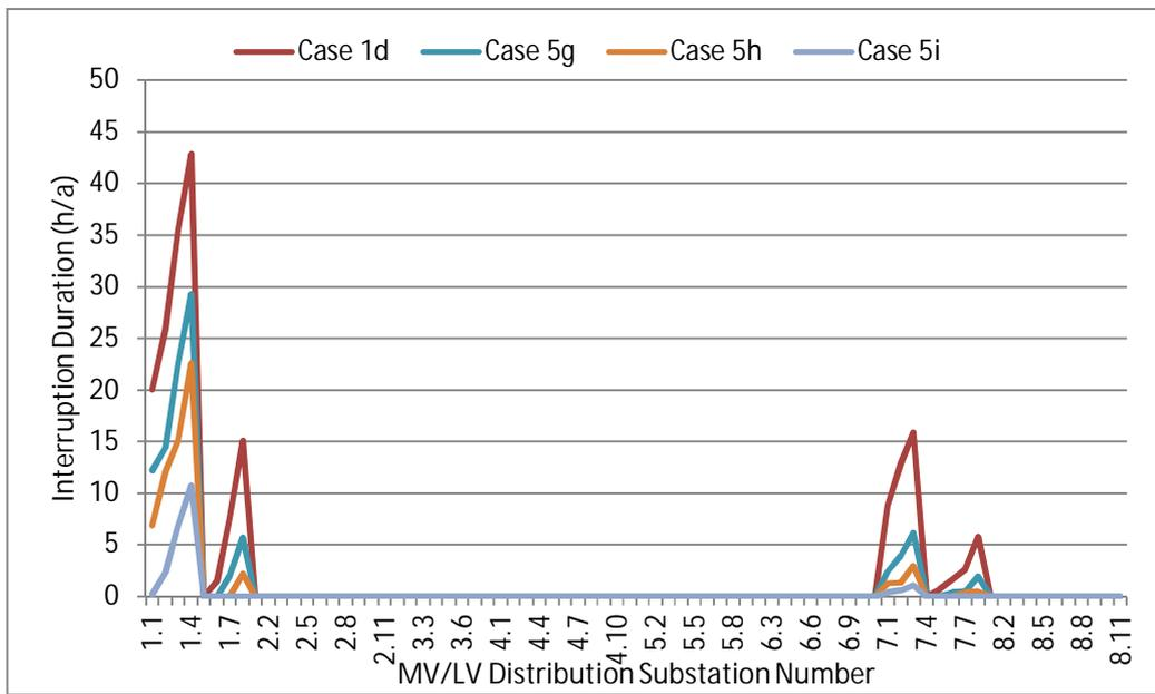
**Figure 5-25: Annual interruption duration for MV/LV substations (Case 5g-5i)**
