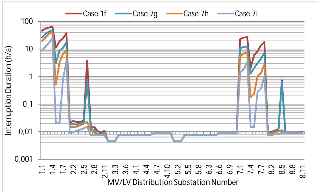
*Figure 5-33: Annual interruption duration for MV/LV substations (Case 7g-7i)*
