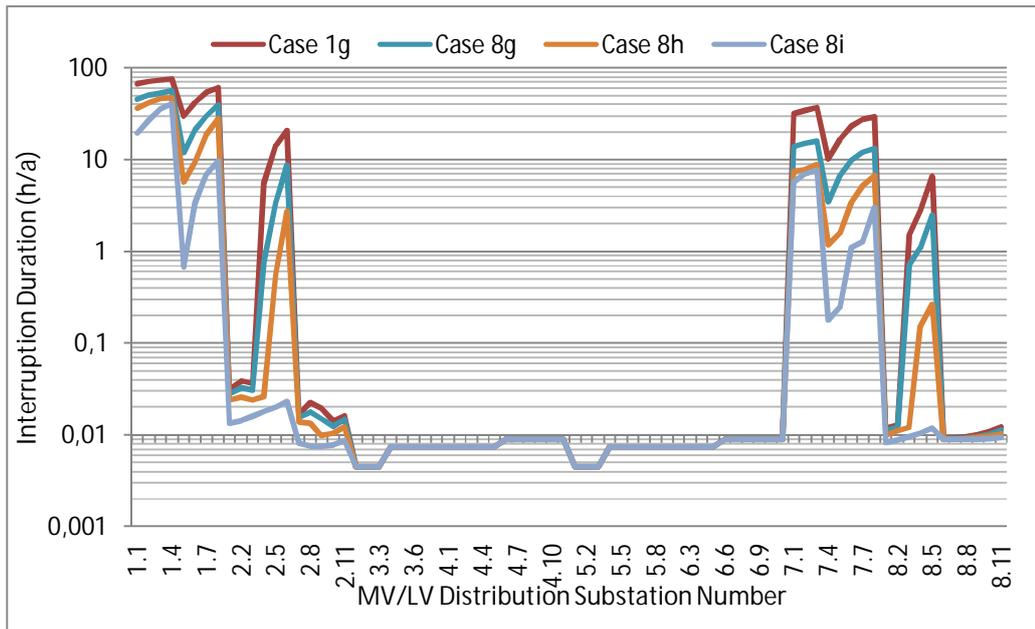
**Figure 5-37: Annual interruption duration for MV/LV substations (Case 8g-8i)**
