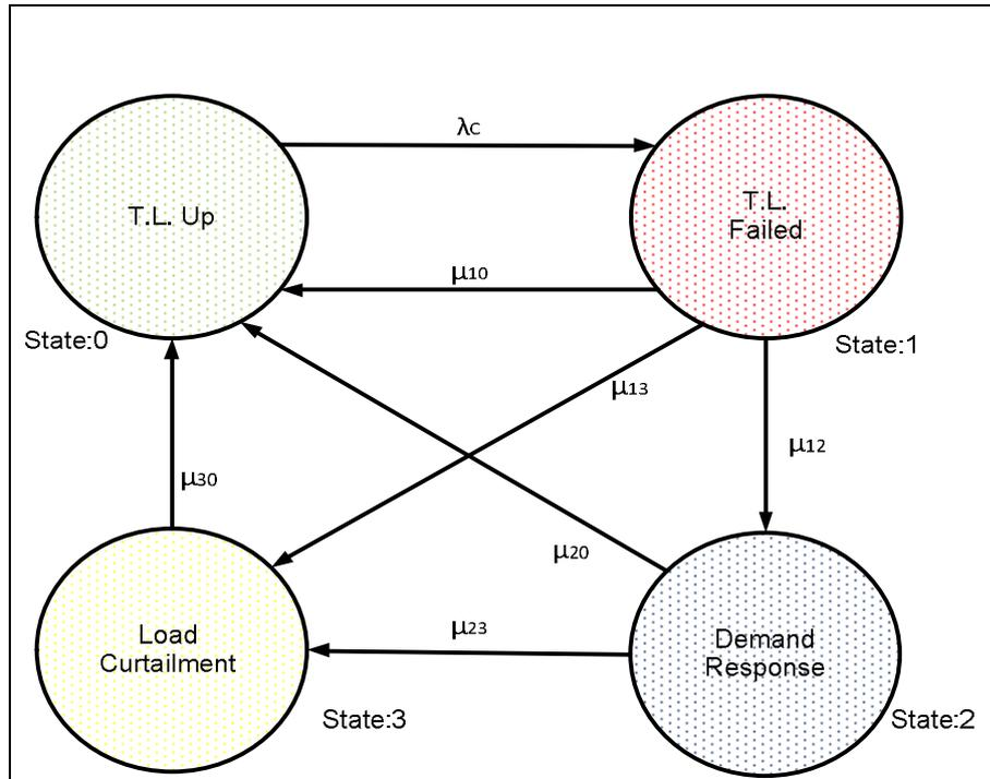
*Figure 4-3: Modified model for sub-transmission line segments.*
