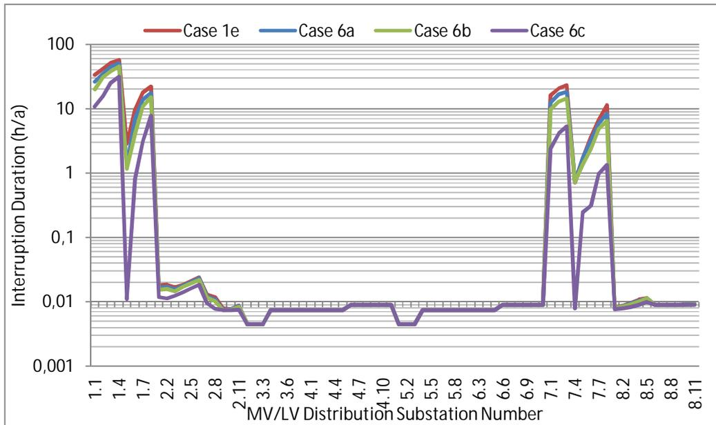
**Figure 5-27: Annual interruption duration for MV/LV substations (Case 6a-6c)**
