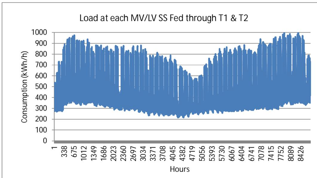
**Figure 5-2: Annual Load profile at each MV/LV substation fed through T1 & T2.**
