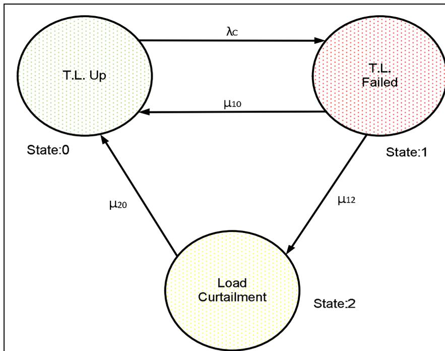
*Figure 4-1: Basic model for sub-transmission line segments.*
