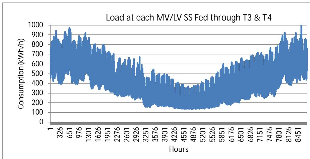
**Figure 5-4: Annual Load profile at each MV/LV substation fed through T3 & T4.**
