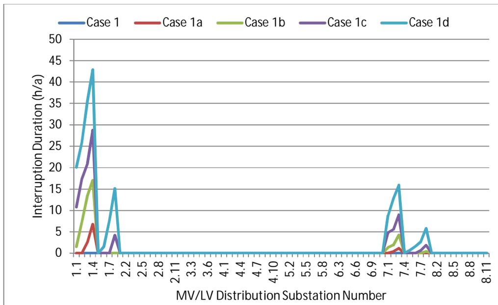
**Figure 5-8: Annual outage duration for MV/LV substations (Base cases 1-1d)**
