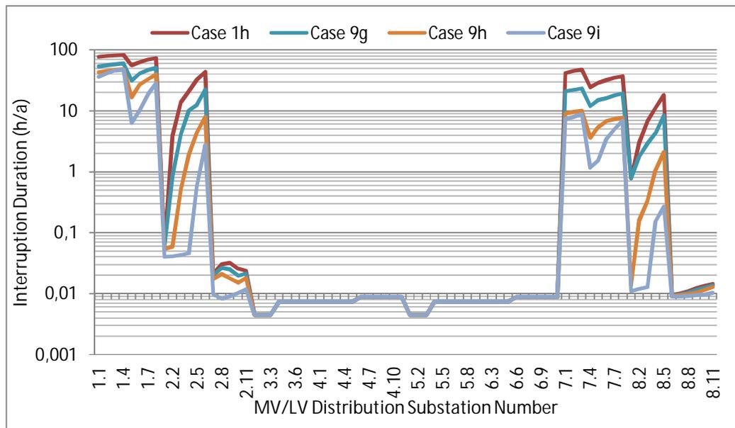
**Figure 5-41: Annual interruption duration for MV/LV substations (Case 9g-9i)**
