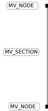
Figure 8.2: A basic topology in DMS 600 internal format. Two components are connected to each other via an MV Section. The electrical characteristics of the connection are represented by a conductor type associated with the MV Section. A special conductor type, BUSBAR , is used to represent connections with zero impedance.
