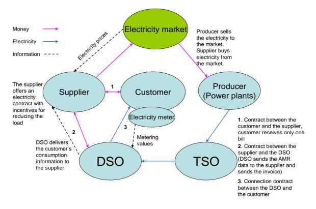
Figure 5.2. Schematic picture of demand response in supplier centric market.
