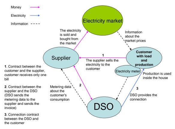
Figure 5.1. Schematic picture of connecting small scale production.
