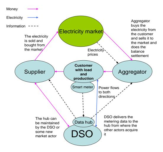
Figure 6.1. Schematic picture of small-scale production with new market actors.
