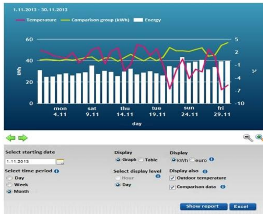
Figure 4.1. Consumption graph in the energy reporting service. An example consumption site presented.
