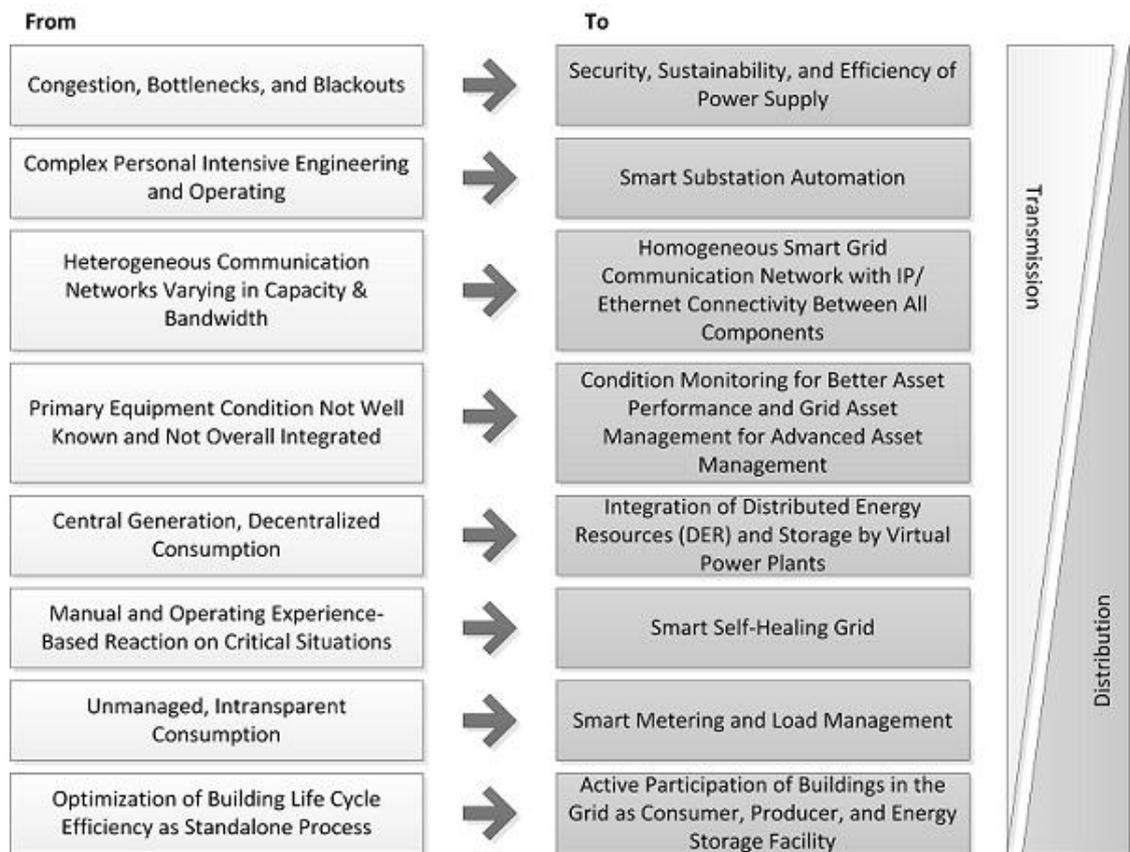
Figure 3 Transforming to Smart Grid [7]
