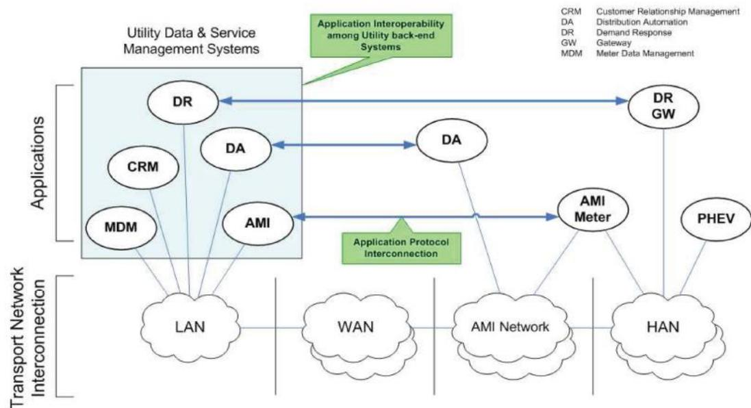
Figure 10 AMI Communication Network Structure
