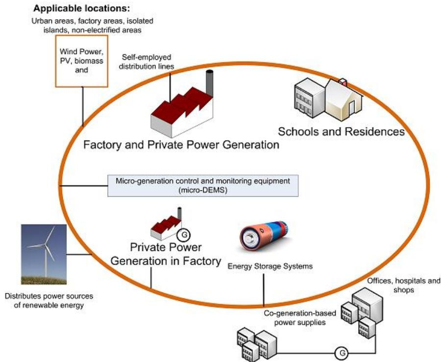
**Figure 18 Microgrid network model**
