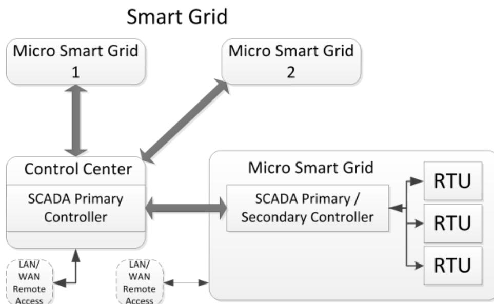
**Figure 14 Proposed Smart Grid SCADA Network Layout**
