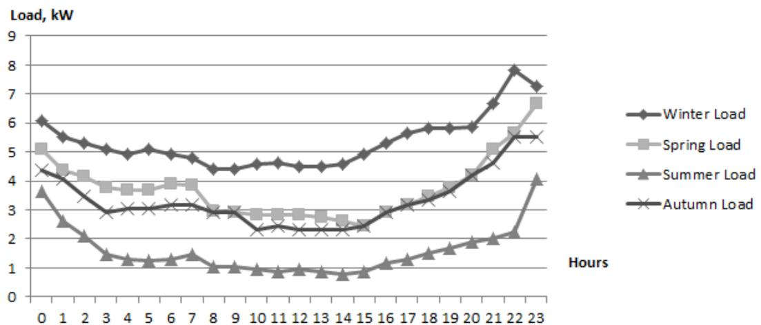
**Figure 34 Load Curves for Detached Houses with Applied Growth Coefficient**
