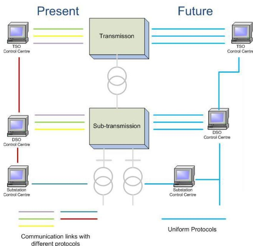
**Figure 13 the Smart Grid Roll-out of Communications Coverage to the Distribution Level [4]**
