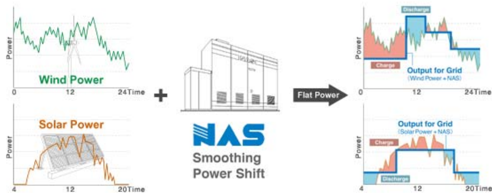
Figure 4-34. NaS system stabilizing intermittent renewable energy [Source: NGK].
