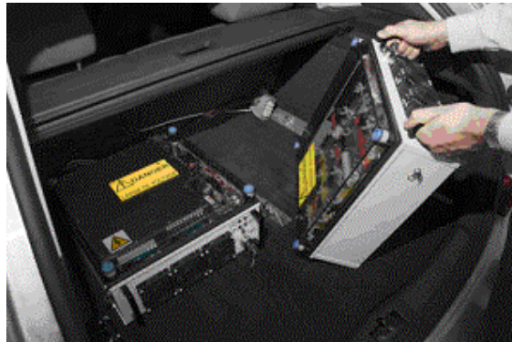
Figure 4-56. PHEV removable battery pack [Source: MIRA & Skoda Fabia].
