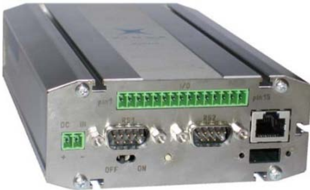
Figure 15. Arctic RTU from Viola Systems connects remote devices to SCADA.
