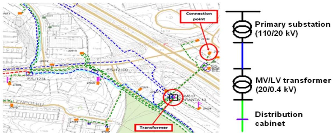
**Figure 6.3.** Grid view and basic principle of distribution arrangement of the case 3.
