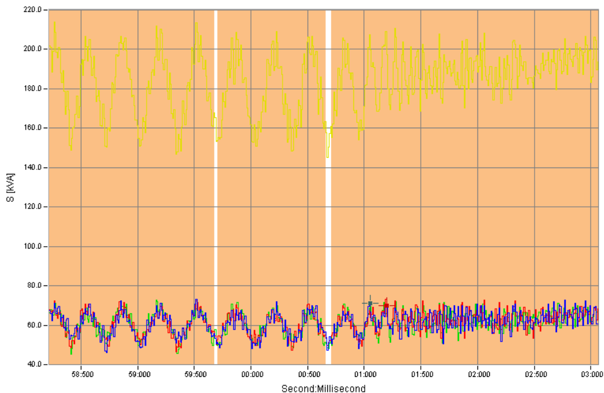
Figure 22. The RMS apparent powers/kVA 28.09.2010 11:27:58 - 11:28:03 with a measurement time of 5 s; L1 = blue, L2 = red and L3 = green and sum of the formers = yellow The recorder has flagged the brown areas of the figure.
