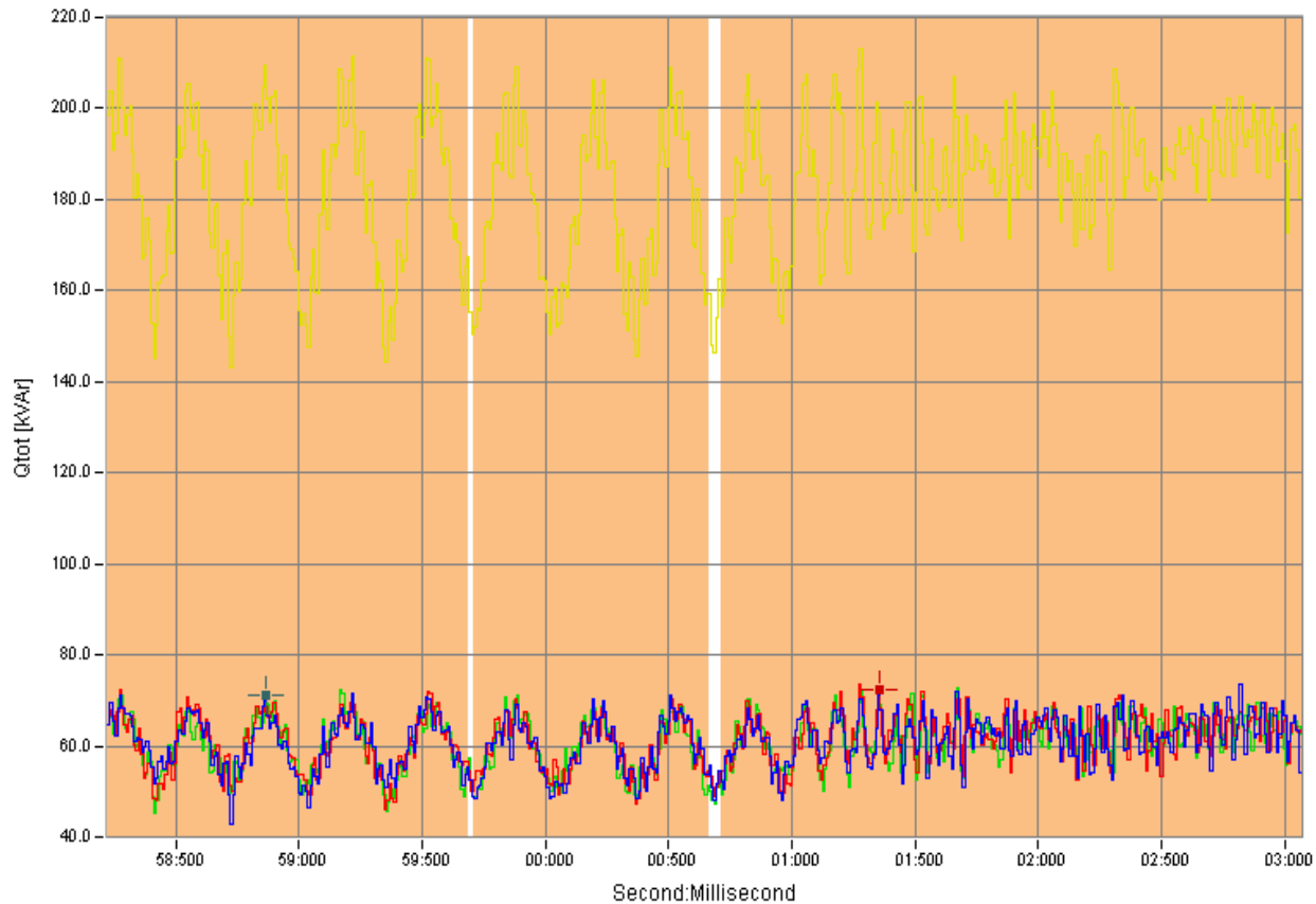
Figure 21. The phase RMS reactive powers/kVAr 28.09.2010 11:27:58 - 11:28:03 with a measurement time of 5 s; L1 = blue, L2 = red and L3 = green and sum of the formers = yellow. The recorder has flagged the brown areas of the figure.
