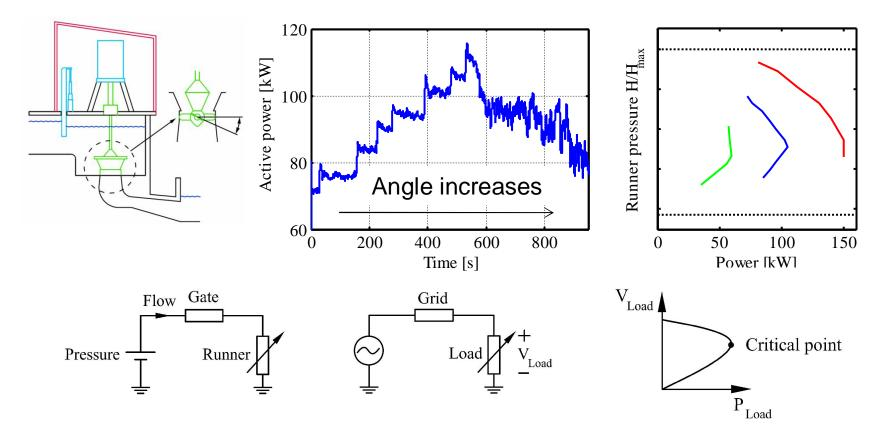
Gate control not possible > use dump load for low load operation
