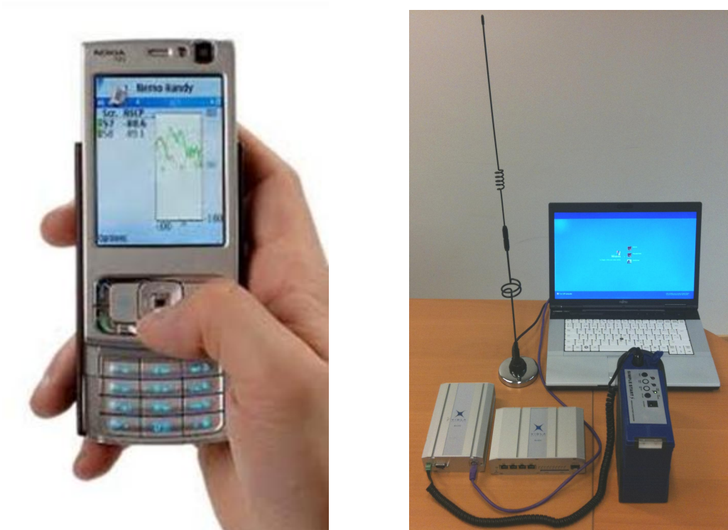
Figure 2. Nemo Handy measurement device was used as typical terminal and Viola System's Arctic EDGE Router and Arctic 3G Gateway for a dedicated RTU.
