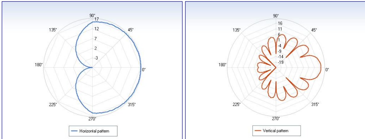
Figure 7. Antenna patterns of Kathrein 80010517.
