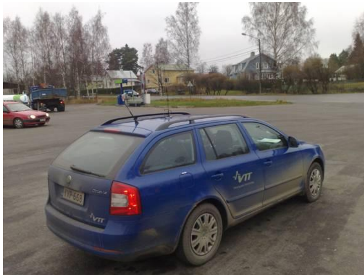
Figure 18. The car used for measurements. The RTU's external antenna is mounted on the middle of the car roof.
