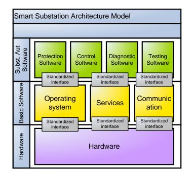
Figure 2. New substation concept [Car10].
